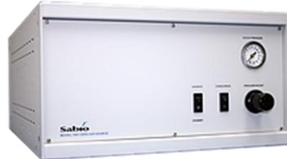
The Model 1001 is equipped with dual coalescing filters and a permeation drier; moisture removal is enabled automatically using adjustable control circuitry or manual purging from the front panel. Additionally, the air source can be controlled by all Sabio calibrators via contact closure or on demand when an optional internal pressure switch is installed.
