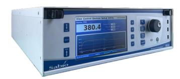
The Multi-gas system is designed to be either sequence based (gases are established, gases are assigned to source input ports, desired dilution flow defined, and output concentrations are established), or the unit can be manually controlled by the operator from the status window. Flexibility, without complicated menu systems or restrictions allow the operator to fully control the calibrator for various applications.
