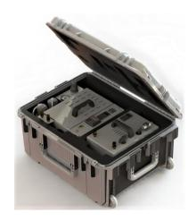
The Model 2020-EXP uses an internal permeation drying system for moisture removal and is coupled with filter canisters for scrubbing NOx, NO, NO2, O3, SO2, and H2S. Optional features such as the internal carbon monoxide (CO) oxidizer, or the internal hydrocarbon (HC/CO) oxidizer, further the Model 2020-EXP's clean air capabilities.
