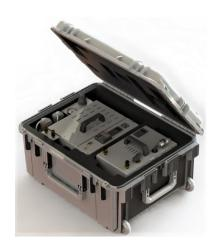
The Model 2020-EXP uses an internal permeation drying system for moisture removal and is coupled with filter canisters for scrubbing NOx, NO, NO2, O3, SO2, and H2S. Optional features such as the internal carbon monoxide (CO) oxidizer, or the internal hydrocarbon (HC/CO) oxidizer, further the Model 2020-EXP's clean air capabilities.
